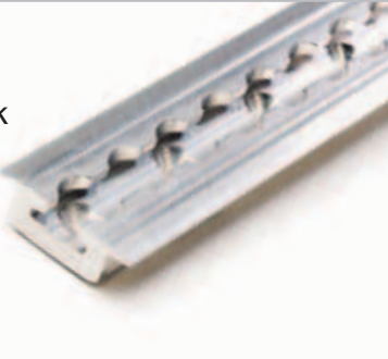
FE751-01-PD2 Medium-Duty Series L Track with Flanges and Mounting Holes Spaced on 2" Centers Material: 6061-T6 Aluminum Weight: 6.2 lb/2.8 kg
