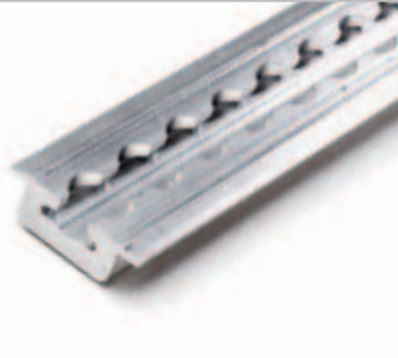
FE751-01 Medium-Duty Series L Track with Flanges Material: 6061-T6 Aluminum Weight: 6.4 lb/2.9 kg
